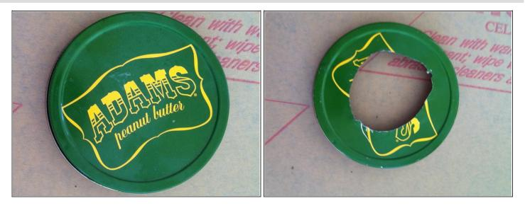
• After machining all of the acrylic parts, take a pair of tin snips and cut out a rough circle approximately in the middle of the peanut butter lid. Make sure the hole's diameter is bigger than 2".
